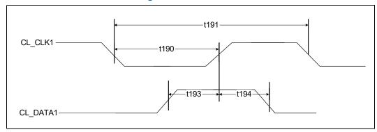
Figure 10-23.Controller Link Receive Slew Rate
