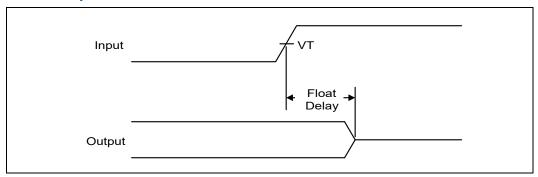
Figure 10-16.Output Enable Delay
